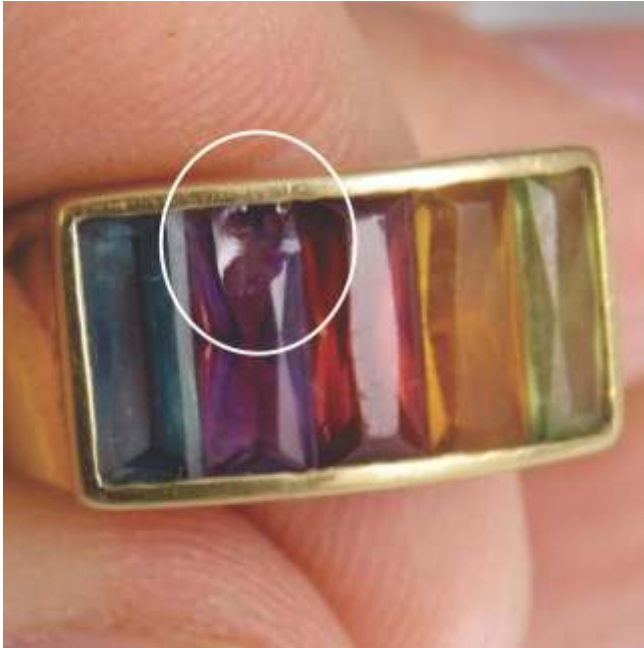
Fig 3.3.7 Stone has got damaged due to rough use of setting tools
