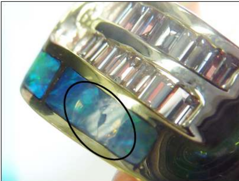
Fig 3.3.8 Soft stone has got cracked and damaged due to rough use of setting tools
