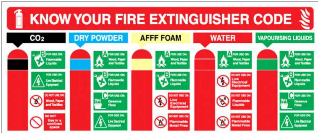
Fig 5.4.2 Know your fire extinguisher code
