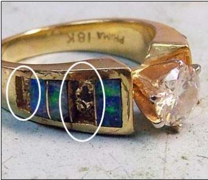
Fig 3.3.9 Soft stone has got completely damaged due to rough use of setting tools
